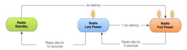
The radio state machine on each device, particularly the associated transition delay ("tail time") and startup latency, vary based on the wireless radio technology employed (2G, 3G, LTE, etc.) and is defined and configured by the carrier network over which the device is operating.
